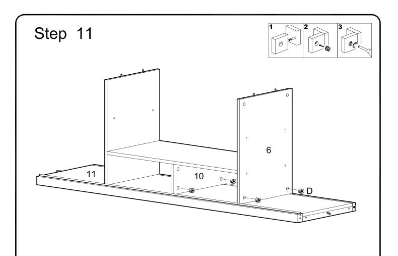
Secure panels (6,10) to bottom panel (11) using cam locks (D). Tighten cam locks (D) with a screwdriver.
